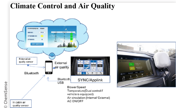
FIGURE 5 Air quality diagram and image of ChemiSense sensor.
